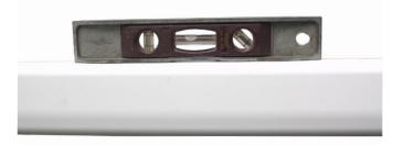
In this example, the wall is to the left. Notice that the bubble is indicating that the arm is sloping down
